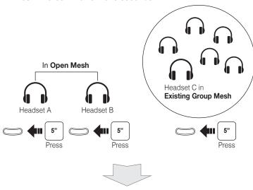
When headsets complete Mesh Grouping, headsets automatically switch from Open Mesh to Group Mesh, and users (A, B) automatically join the existing Group Mesh.
