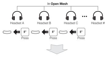
When headsets complete Mesh Grouping, headsets automatically switch from Open Mesh to Group Mesh, and users automatically create and join the Group Mesh.
