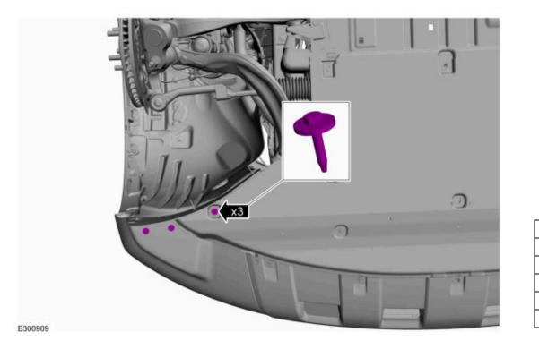
6. Remove the screws. *Torque*: 22 lb.in (2.5 Nm)
