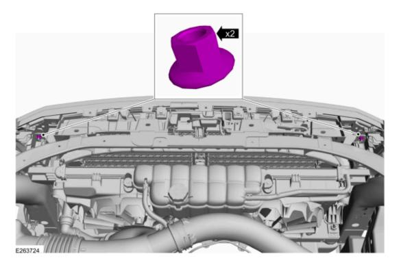
7. Release the clips and remove the radiator grille.
