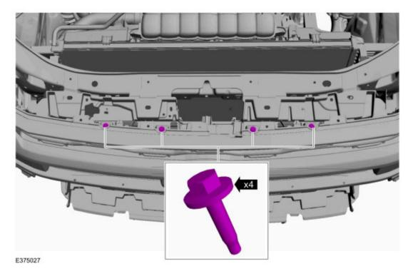
6. Remove the radiator grille mounting nuts. *Torque*: 53 lb.in (6 Nm)
