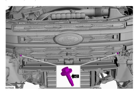
5. Remove the radiator grille mounting upper screws. *Torque*: 28 lb.in (3.2 Nm)
