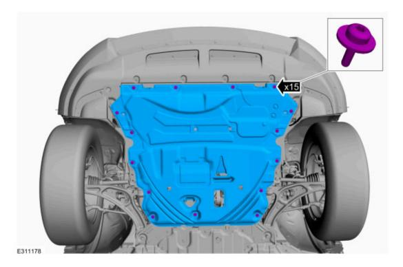
5. Remove the screws. *Torque*: 18 lb.in (2 Nm)
