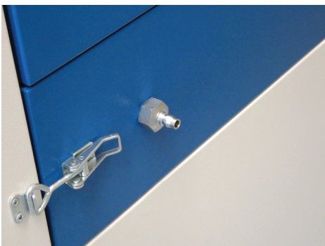
Simple air supply to power filter cleaning
