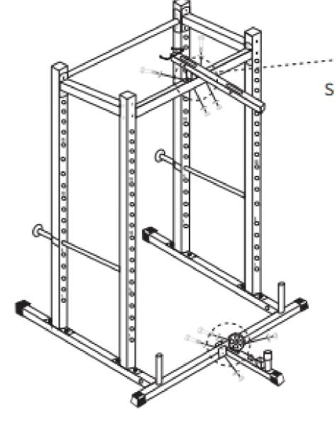
Secure top and bottom pulley brace of lat pull down to crossbars of the rack.
