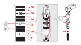
The height of the offset number (shown in the drilling report) on the driver is determined either by the line in the middle of the number (see 'a') or by the line in between the laser marking (see 'b').
