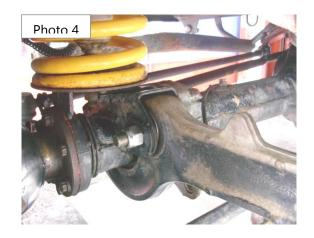
Wheel-align the vehicle before the job is started and note castor settings
