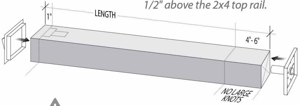
Inspect the post to make sure there are no large knots in the lower 4"-6" of the post. Knots will prevent the tube from cutting into the post and in some cases causing the post to crack.
