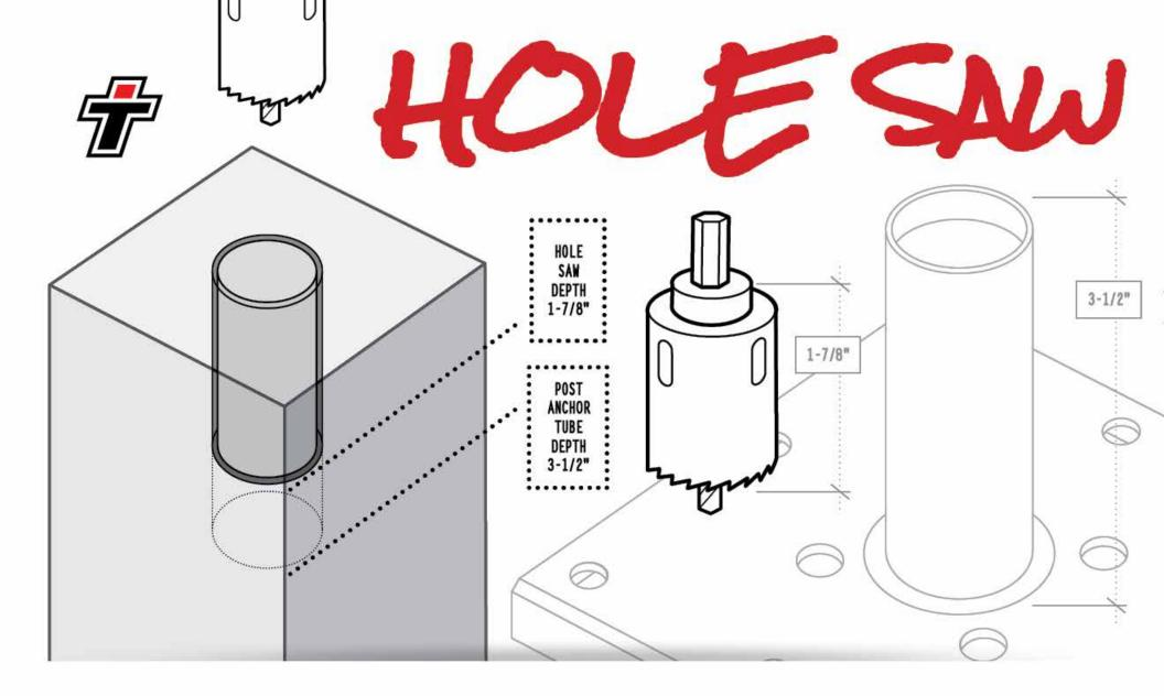
Right away you will notice that the hole saw is **shorter than the tube** which is at least **3-1/2" long**. That is just fine because you are going to **plunge the hole saw straight down as far as it can go.** Pull the hole saw out and notice the circular **kerf** cut that is left behind and the **wood plug remains in place.**
