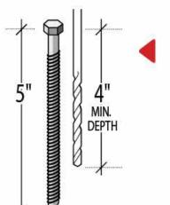
For 3/8" lag screws, use a 5/16" speed bit and make sure it extends at least 80% of the length of the screw. For a 5" screw, pre drill to a minimum depth of 4".
