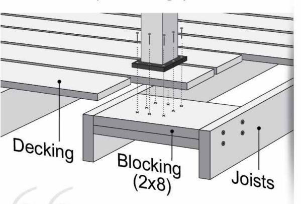
A 2x8 is a nice size because it easily exceeds the 5" dimension of the 4x4 post anchor and also that of the 6x6 post anchor. Furthermore most decks are framed with 2x8 joists so there is usually lots of scrap lying around to use for blocking.
