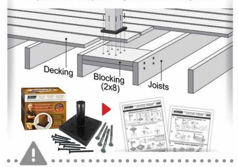
Follow the instructions provided with your kit for installing the post anchor to the posts. Bracing between the posts and rafters is recommended to stop the pergola from racking. Some construction designs may be sufficient and not require bracing.
