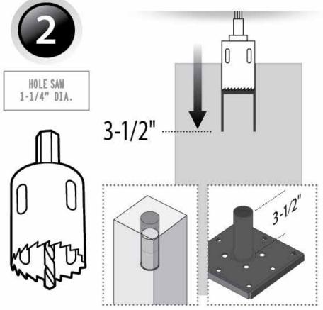
After the first pass with the hole saw, use a 1-1/4" dia. Forstner bit to remove the core left behind and drill down to a depth of 1-5/8" from the bottom of the post. Be sure to *clamp* the post into a *vice* or against a *bench* when using the Forstner bit and go slow and carefully as the Forstner bit can kick back in hardwood.
