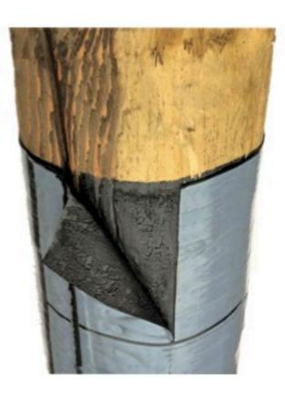
Polesaver full barrier sleeve peeled back to show air and watertight bituminous sealant on the pole surface in-between the outer sleeve and the pole
