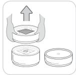
Gently remove the top unit and disassemble the remaining power filter modules.
