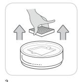
Safely remove the ceramic filter from the power filter module.
