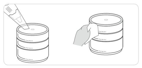
Remove any visible dust from the unit's surface. Gently wipe with a clean soft cloth. DO NOT USE the following products: benzine, thinners, polishing powder or other solvents.
