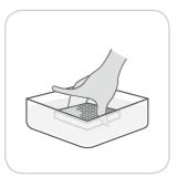
Lay the filter in a bowl filled with warm water. Let it soak for 30 minutes.
