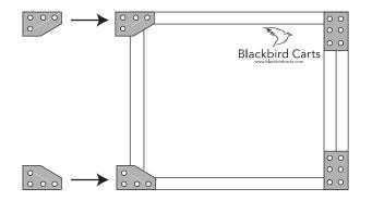
2. Lower 40-inch verticals on to back side of Equipment Box. Make bottom of Vertical Rail flush with bottom of box. Tighten Bolts A through D
