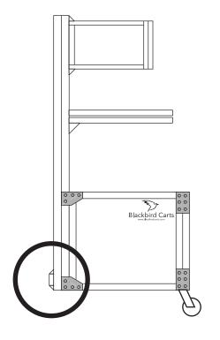
4. Place assembly on all 4 wheels on the floor. Then, slide mixer shelf down from top and follow with Upper Monitor Box. Tighten bolts to secure in place.
