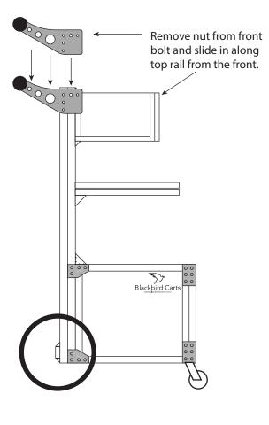
5. Slide Top Handle Assembly down onto outside of vertical rails and align top holes with top rails of the Monitor Box. A T-Nut has been pre-installed in top rail of Monitor Box for forward most bolt.
