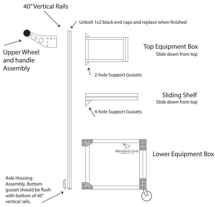
1. Slide 90 degree brackets on to top, back side of Lower Equipment Box. Make flush with back of top rail.
