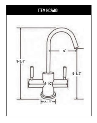
Max Counter Thickness 2" Recommended Installation Hole: Cold Only 3/4 to 1" Hot Only 1–3/8" Hot & Cold 1–3/8"
