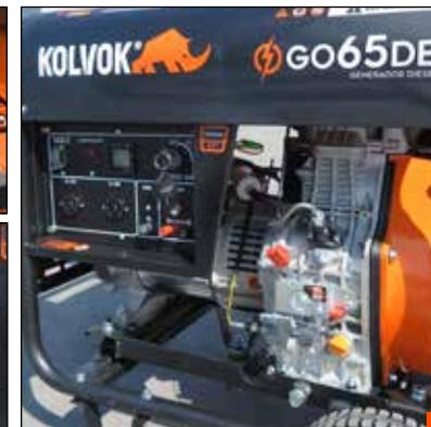
Interruptor General 2 salidas AC230V Cargador DC 12V / 8,3A
