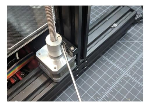
Turn your printer onto its side so that you can access the two screws on each side beneath the vertical rails. Remove these screws and set the rails aside.
