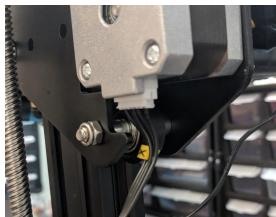
Twist the lead screw to move the X carriage rail up, all the way to the top, and detach it from the lead screw. Carefully remove the X carriage from the vertical rails. Set it aside.
