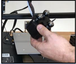
Press on the plastic retention ring towards the hot-end and pull the Bowden tube out of the hot-end.
