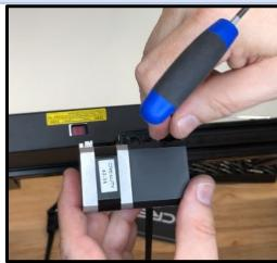
Attach the Y end stop switch wire to the end stop switch.
