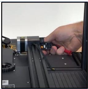
Disconnect the Y axis end stop wire connector from the inside of the cover
