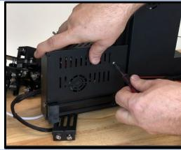
Attach right side assembly to Y axis center beam
