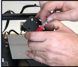
Remove the other end of the Bowden tube from the extruder.
