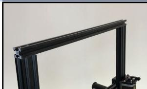
Attach a small clamp to the top cross bar and the X axis to hold them in position where the X axis is near the top. The clamp should be attached to the left side near the motor.
