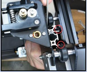
Slide the X axis assembly back down onto the vertical frame members; support the carriage with the filament spool holder.
