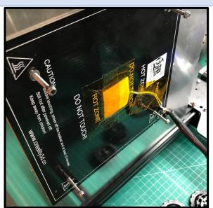
Tighten the M4 lock nuts against the washers and stock heater plate.
