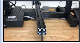
Locate the Y carriage plate, and fit it to the Y axis 4040 extrusion, taking care not to damage the wheels. Ensure the narrow corner faces the back/left of the printer. Slide the Y carriage towards the middle of the printer.
