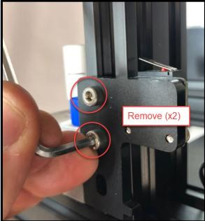
Remove the Y axis belt tensioner wheel
