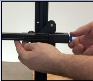
Attach the top cross bar with four M5x20 screws
