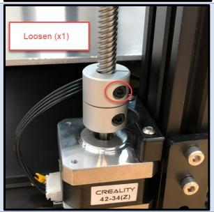
Carefully pull upwards until it disengages from the coupler.
