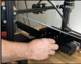
Attach the levelling wheels.
