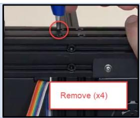
Remove power supply mounting screws from underside of right support beam.
