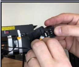
Attach the Y end stop switch cover. Take care the wires do not get pinched between the cover and the motor mount.
