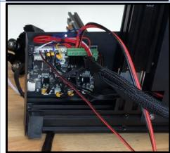
Remove the Y motor and end stop cable from the control board plugs. They may be secured with hot glue, therefore, use a tool (not a knife) to remove the glue.
