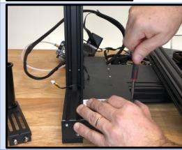
Feed Y belt through Y axis tube, ensure the belt does not become twisted.
