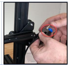
Attach the belt tensioner cover to the X axis. The front screw is a counter sink screw; the rear is a round head screw.
