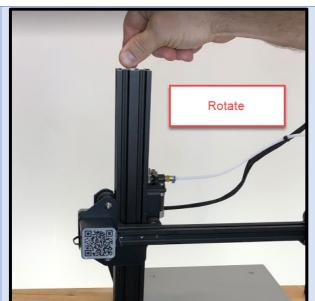
Place the filament spool holder under the x axis bar on the left side of the frame.
