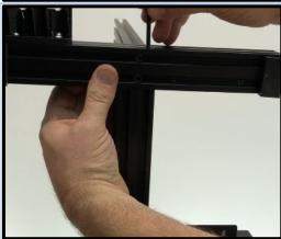
Attach Y axis 4040 beam to center cross beam. The long end will face towards the front.
