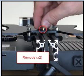
Slide the Y carriage plate towards the front of the Y axis and remove the Y carriage plate assembly
