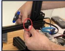
Locate the X axis belt and feed the left end through the motor pulley cover, around the pulley, and back under the X axis bar. This part is tedious! We find it makes it a bit easier if you use a tool to guide the belt through the small gap at the end of the X axis bar.
