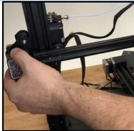
Support the X axis assembly with the filament spool holder
