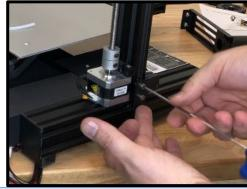
Locate the utility drawer support bracket. Use the included M5 screw and T-slot nut to attach to the center cross beam. Hold pressure on the bracket against the drawer side, tighten screw to hold drawer in place.
