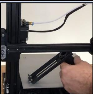
Loosen the top grub screw in the Z motor coupler
