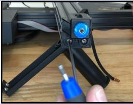
Attach the belt ends to the Y carriage plate
