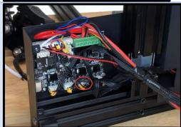
Pull the Y motor and end-stop wire towards the motor to lengthen it.
