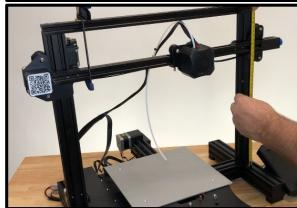
Once the left and right sides are equidistant from the bottom frame members, tighten the two screws on the back of the right-side X axis carriage.
