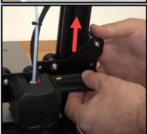
Slide the left side of the X axis assembly up to the top of the left vertical extrusion and carefully remove the X axis assembly from the Z vertical extrusion.
