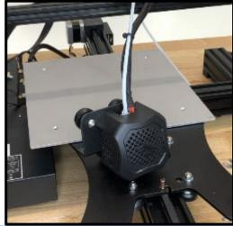
Loosely attach right side plate to X axis using one screw.
