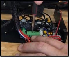
(Stock bed heater only: I attached the black to the left terminal. It does not matter which terminal; however, you should attach it the same way it was before you detached it)
