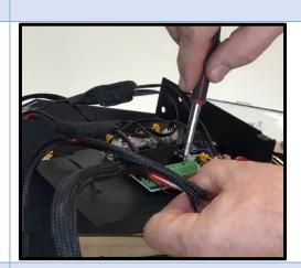
Remove the Y motor and Y end stop connectors from the control board.
