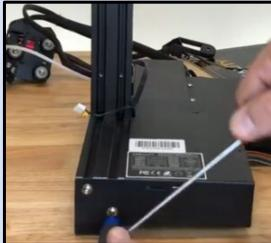
Remove control board bottom cover screws (3)
