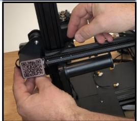
Slide nozzle assembly onto the X axis bar from the right side; ensure the belt is positioned below the wheels. If the assembly will not clear the right gantry carriage, loosen the gantry carriage screw on the back.
