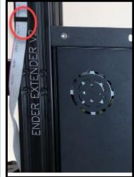
Attach top control board cover screws (2)
