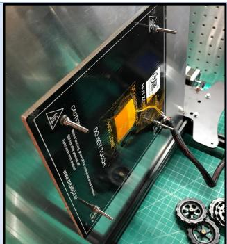
Position the levelling springs on the levelling screws.
