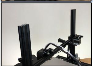
Hold the X axis assembly and remove the clamp(s). Carefully slide the X axis up to the top of the vertical Z axis frame members.
