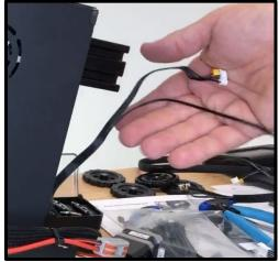
Using the included Y motor extension wire, connect the existing motor cable to the extension cable. Connect the Y motor extension wire to the control board.
