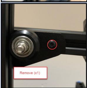
Remove the X Axis Belt Tensioner cover and bearing holder.
