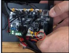
Attach the control board to the left / bottom frame member
