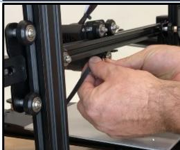
Tighten the X belt tensioner, ensure the belt is not over tightened.
