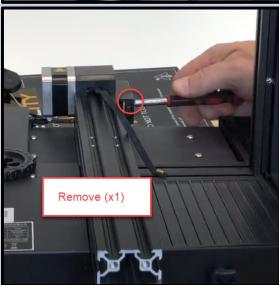
Remove Y axis end stop cover. It is a snap fit, so take care while removing.
