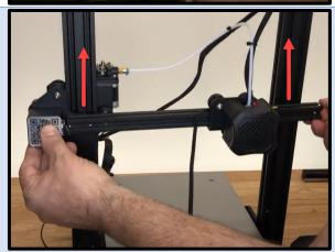
Place the X axis assembly on the printer bed and locate the two screws embedded under the extruder bracket. Use the short end of the hex key tool to loosen the screws, then use the long end through the holes in the extruder bracket to remove the screws.
