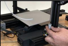
Tighten the lead screw in the Z motor coupler. Use short side of allen key tool to tighten.
