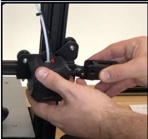
Disengage both ends of the X axis belt from the underside of the nozzle carriage plate.
