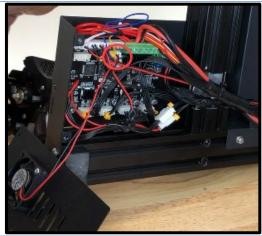
Attach LCD cable to control board. The LCD cable has a proper orientation; on the control board side, the square key on the connector is on the inside facing the cable.
