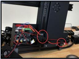
Reattach bottom control board cover fan wire to control board.
