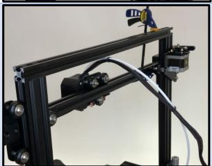
Measure the distance between the X axis bar and the left and right bottom frame member; adjust the right side up or down, holding the motor side in place.
