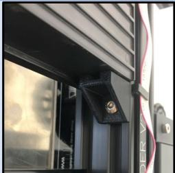
Attach front support (3D printed part) to underside of Y axis. Adjust the location to suit your needs. Adjust the height to make contact with your table by squeezing or stretching the part length-wise.
