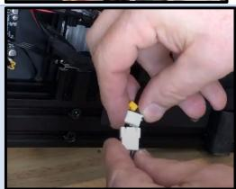
Take care to route the wires through the cutout. Use zip ties and electrical tape to secure the wires and to protect them from the edges.
