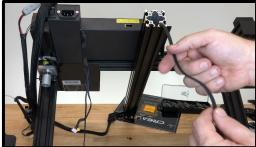
Loop the Y belt over the Y motor pulley through the opening.
