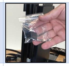
Position plastic bracket on the Y axis center support beam near the power supply flange.
