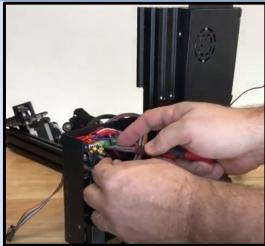
Remove LCD cable from control board
