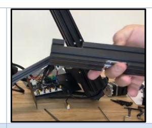
Locate the heated bed thermistor wire connector and unplug it from the control board.
