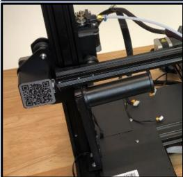
Remove the nozzle cover to gain access to the Bowden tube retention ring. The cover is held in place by two small screws, and two small plastic notches that act as a hinge. Take care not to break the plastic parts.
