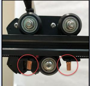
Carefully slide the carriage plate upwards and remove from the vertical extrusion.
