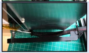
Attach the aluminum plate stack and screws through the springs and carriage plate.
