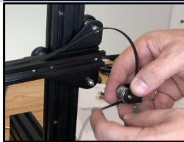
Attach the pulley into the X belt tensioner cover
