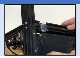
Re-attach the four side mounting screws Locate the power supply support bracket 3D printed. Included in the bag is an M5 screw, M5 t-slot nut, and an M4 screw.
