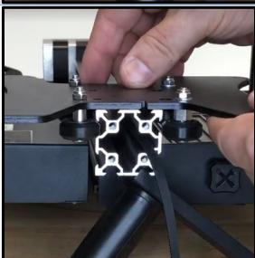
Remove Y axis end stop cover screw
