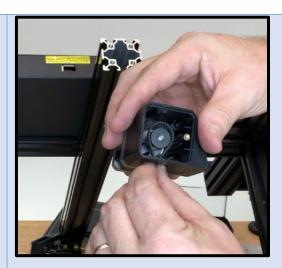
Attach the Y motor to the end of the Y axis.
