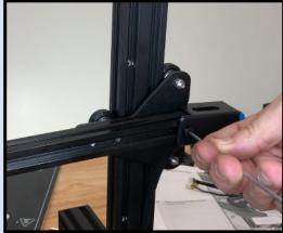
Attach the belt ends to the nozzle carriage
