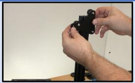
Attach the left side bracket and X axis beam to the left vertical beam
