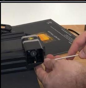
Disconnect the Y axis motor wire
