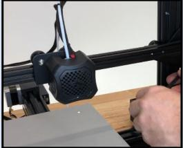
Loop the X belt through the pulley assembly
