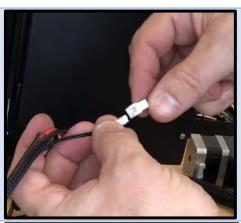
Attach the end of the heated bed extension wire to the control board. The polarity of the stock heat bed connection is not important. However, the Creality wiring diagram suggests the positive wire (red) should connect to the left terminal. Ensure the black wire is close to the red wire of the power supply line.
