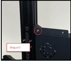
Tighten the M5 Screw to secure the power supply.
