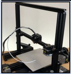
Insert the lead screw into the brass nut and turn it until it reaches the Z motor coupling. Insert the lead screw into the Z motor coupling.
