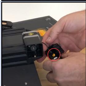
Remove the Y axis motor mount
