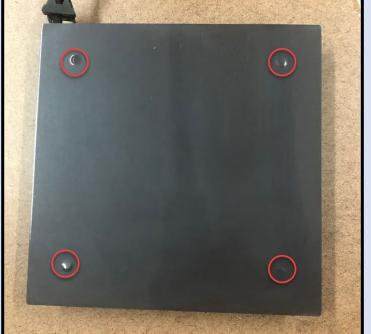
Position the new larger plate atop the stock heated build plate.
