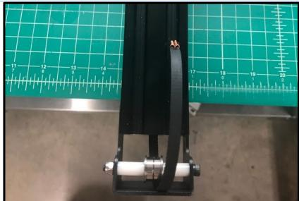
Attach the Y motor mount to the opposite end of the Y axis, feeding the belt through the motor mount belt hole, and over the pulley. (Ender 3 Pro shown)
