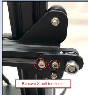
14 Disassemble X axis
