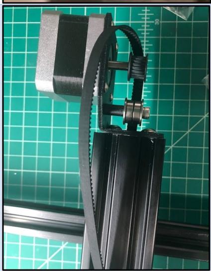
7 Attach the end of the belt to the carriage plate as shown.
