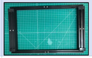
Use your carpenter square to ensure the frame is square in each corner before tightening the screws. Take your time and double check each corner.
