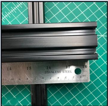
9 Use the square tool to ensure the Y axis is square to the cross members and tighten the frame screws.
