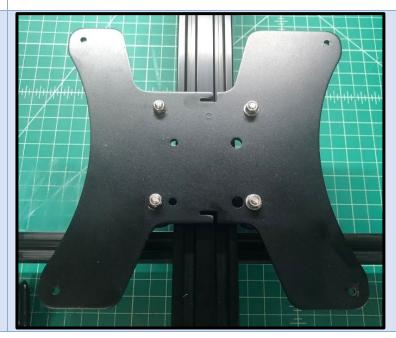
4 Attach the Y belt tensioner to the Y axis, feeding the end of the belt through the tensioner and onto the bearings. (Enter 3 Pro shown)
