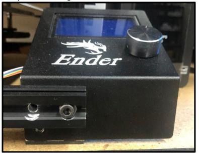
Example control box mounting on a Non Pro kit:
