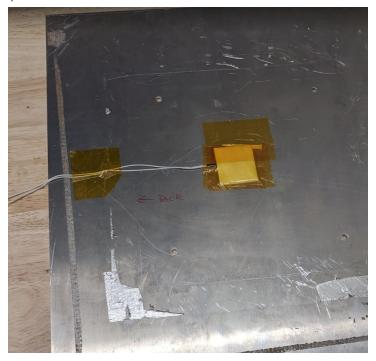
Now you're ready to attach the very sticky side of the heat pad to the plate. Warning: Once installed, you are not likely to get it removed. Remove the paper from the heat pad and carefully center the heat pad over the holes and corners, with the wires pointing in the same direction as the thermistor wires. TIP: You might have some luck by inserting the bed screws through the holes, with the plate on the table as show, screws pointing up, might help guide the pad correctly.
