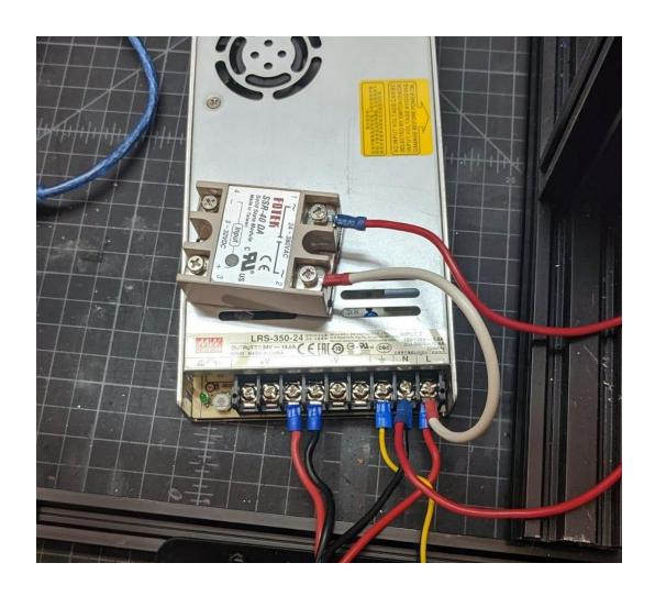
The final arrangement of the wires are shown below. The red wires at the bottom right go to the heat pad.
