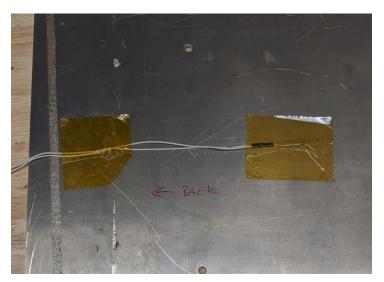
Make sure the thermistor head has good contact with the heat plate. Cover it with one layer of Kapton tape, then follow up with the layer of insulation padding and the remainder of the tape.
