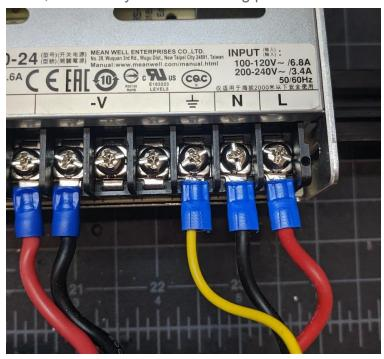
The current revision of this kit includes a short piece of wire (either red or black, depending on what we have on hand). You can connect the bare wire to the screw terminals on the power supply and SSR, but it is highly recommended that you use crimp style terminals. If you use crimp terminals, crimp them onto both ends of the wire. You will also need to crimp terminals onto the wires coming from the heat pad. I prefer the open terminals such as these:
