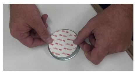
Press the adhesive pad hard against the mounting disk for proper adhesion.
