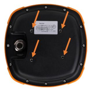
**STEP 2:** Screw the 1" extension into the magnetic mount and then to the mount plate.
