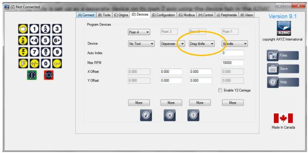
Once the drag knife device is set up any number of tools can be assigned as required to accommodate the different knife lengths and offsets.
