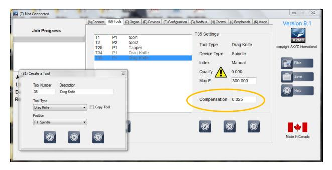
This example is using the Collet style drag knife. The light duty drag knife is similar except that it is set up as "drag knife" in the devices tab as well.
