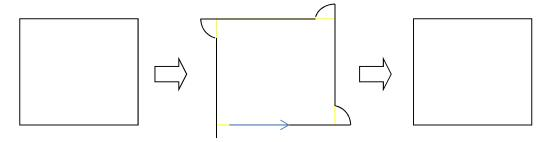
The left diagram is the desired cut path described by the NC file. The A2MC will use the drag knife compensation to create the path shown in the center diagram. The actual cut output is shown on the right.
