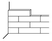
Be sure to imagine how you want the planks to appear prior to installing. There is no need to line up the seams. In fact, it is recommended that you offset the seams for a better appearance.
