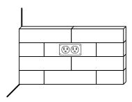
It is recommended that you safely install the boards just under the housing of your light switches or outlets and then tighten the housing onto the boards. This will allow for any covers to install flush on top of the housing and boards.
