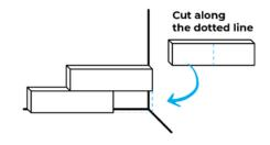
b. Expansion Gap: It is recommended to leave a minimum 1/8"-1/4" gap around the edges of the installation area, and between butt joints to allow for natural expansion and contraction of authentic wood products.
