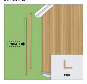
c. **Going Along The Roof:** Install the L trim on the edges of the roof, and attach using screws.
