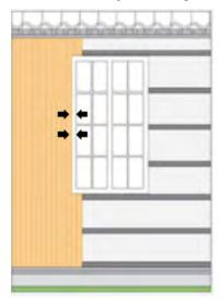
b. Leave a gap of at least 1/8" (3mm) between the board junctions.
