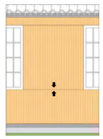
c. Measure and cut the last piece to fit so there is no overhang or excess material.
