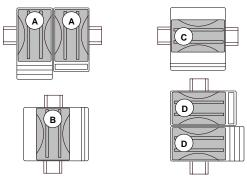
For IC200MDL240 and BXIOIA16120 modules that are mounted horizontally (C, D) on the DIN rail, no derating is required at 120VAC. Deratings at 132VAC are shown below.
