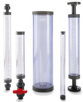
**Griffco** calibration cylinders are designed to enhance the performance of chemical feed systems by providing a verification of the flow rate of the chemical feed pump. Robust construction of clear PVC with an easy to read graduation in mL and gph. Available in three models: EZ-Clean, Vented, and Open Top; and in 15 sizes: 100 mL through 40,000 mL as detailed here.
