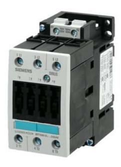
CONTACTOR, AC-3 11 KW/400 V, AC 110 V 50 HZ / 120 V 60 HZ, 3-POLE, SIZE S2, SCREW CONNECTION
