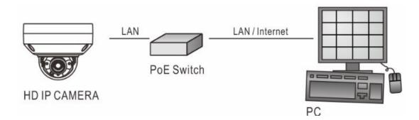
(3). Use PoE power injector and network switch connected to the network.
