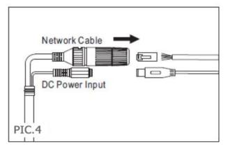
• Connect the RJ-45 Ethernet cable with a waterproof connector
