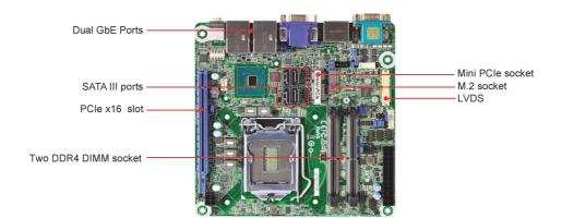
WADE-8211 is based on Intel® Q370 chipset and Desktop processors including Intel® 8th Gen Core™ i3/i5/i7 SKU. This board supports DDR4 ,PCIe 3.0, and SATAIII. Those fratures help you to build high performance and stabile system.
