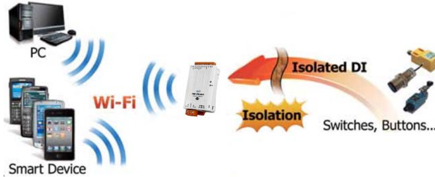
Figure 4-1: tWF + PC/Laptop/Smart Device application architecture
