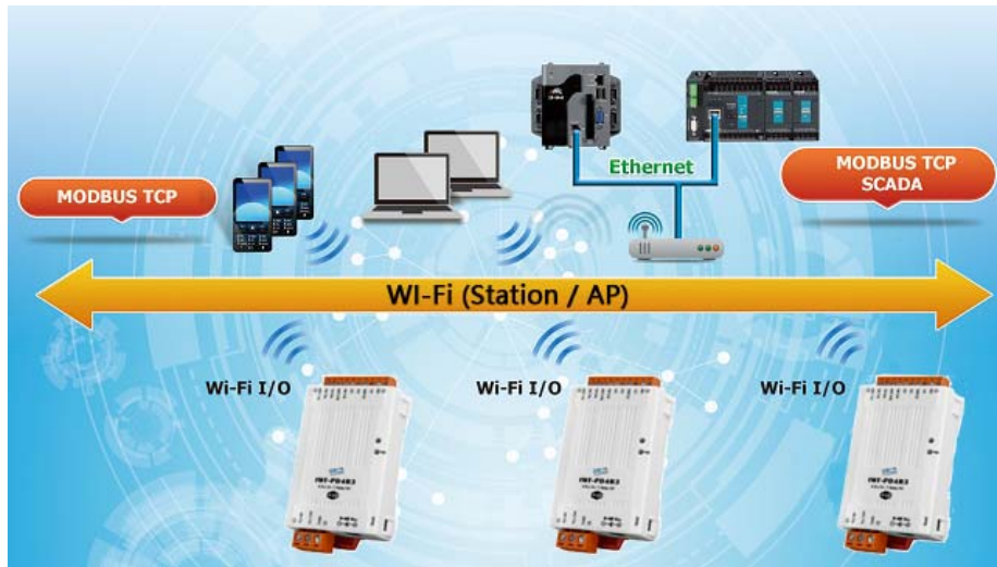
Figure 1-1: Application architecture for the tWF series
