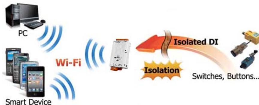
Figure 4-1: tWF + PC/Laptop/Smart Device application architecture
