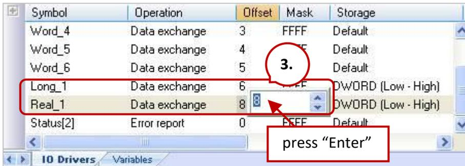
**Note:** Two Modbus addresses are required for 32-bit data.
