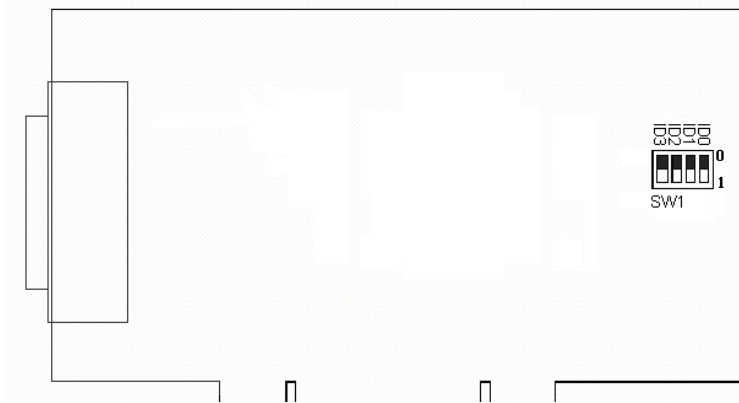
Figure 3.5: Location of DIP Switch on PCI-1758UDI
