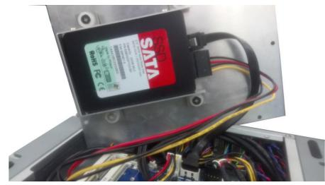
Step 3: Unfasten the <u>4 screws</u> on the HDD/SSD bracket.
