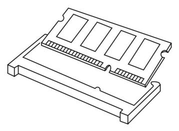
Step 2: Firmly insert the SO-DIMM into the slot until the retaining clips at both ends fully snap back, and the SO-DIMM is properly hold in place.
