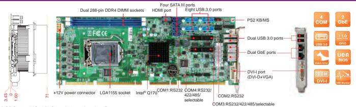
ROBO-8113VG2AR-Q170 is based on Intel® Q170 chipset and desktop processors. Built with flexible PCI express expansions, ROBO-8113VG2AR is suitable for Medical, Industrial automation, and Digital Signage application.
