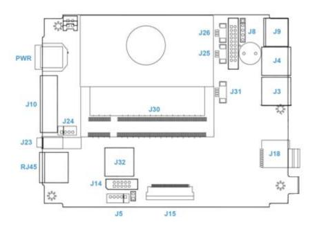
Fig 2-1 PEX CPU Board
