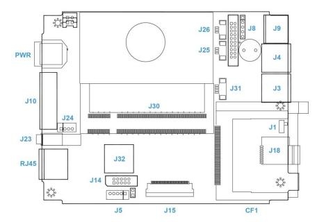
Fig 2-1 PDX3 CPU Board
