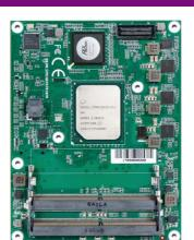
Portwell PCOM-B701 is designed with Intel® new Atom™ processor with brand new Type 7 pin definition. It's built in with 10GbE Ethernet KR interface and DDR4 ECC SO-Dimm support which provide high CPU computing, excellent Ethernet performance. Extend PCIE Gen3 ports in PCOM-B701 can support high speed IO card for more applications. In the meantime, it's compatible with Type 6 carrier.
