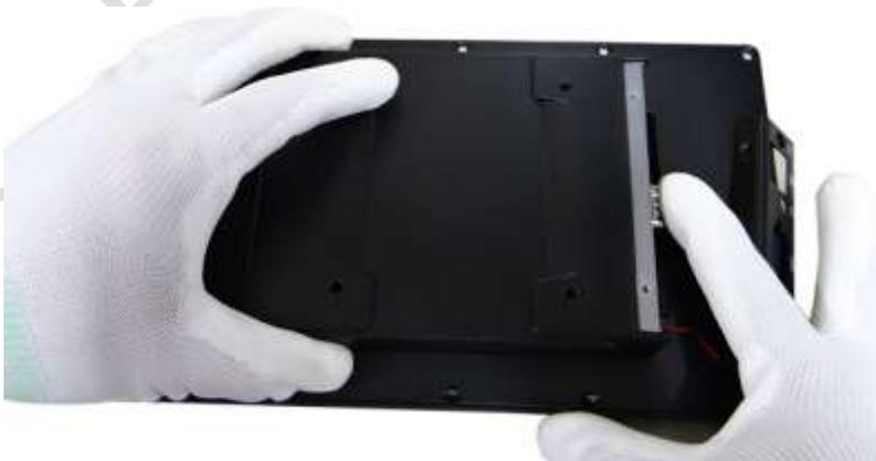
5. Remove the screw of M.2 Slot.
