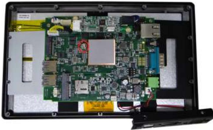
6. Plug M.2 2242 Storage on M.2 Slot and lock the screw back.
