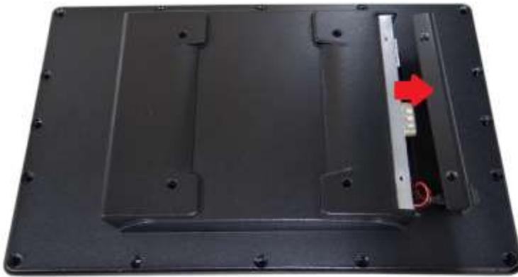
4. Pull up and remove the rear cover.
