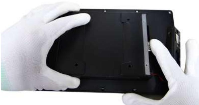
5. Remove the screw of Mini-PCle Slot.
