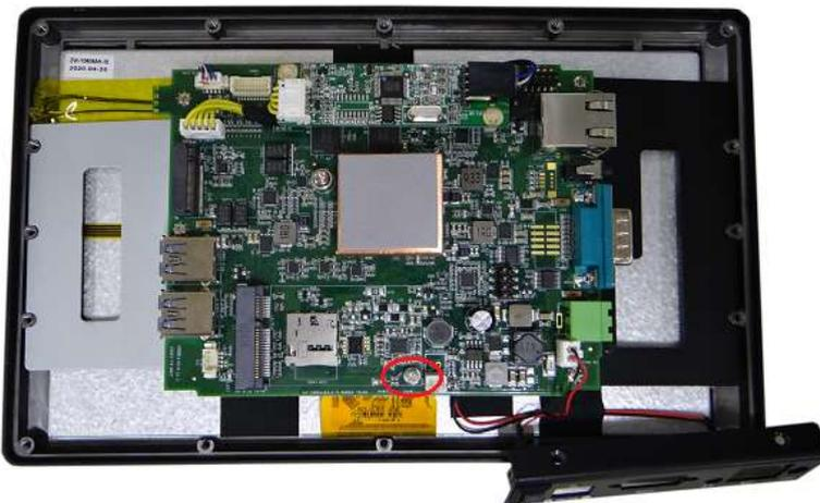
6. Plug Mini-PCle Module in the slot and lock the screws.
