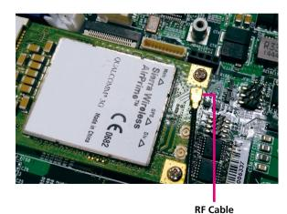
4. Connect the external antenna to the antenna jack.
