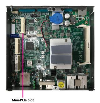
2. Insert the Wi-Fi module into the mini-PCI Express slot at a 45 degree angle until the gold-plated connector on the edge of the module completely disappears inside the slot.
