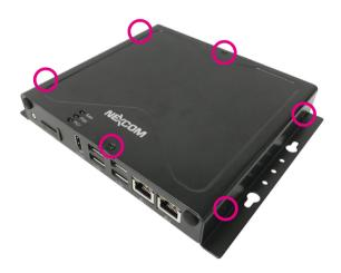
2. With the screws removed, lift up the cover and remove it from the chassis.
