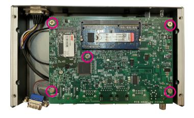
2. Remove the four screws from the front cover.
