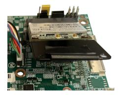
6. Push the module down and secure it with a screw that was removed from step 4.
