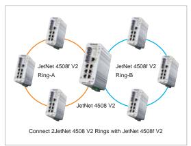
rings into a line or into multiple directions. In addition to extensibility, MultiRing TM has great diversity of various ring technologies. When MultiRing TM enabled, JetNet 4508f V2 can connect RSR rings, TrunkRing TM and a Super Ring together and simultaneously provide more Fast Ethernet Ring connectivities. This provides extensibility to new technologies while keeping the great backward compatibility.
