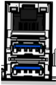
Figure 3-34: RJ45 & USB 3.2 Gen 1 Connector
