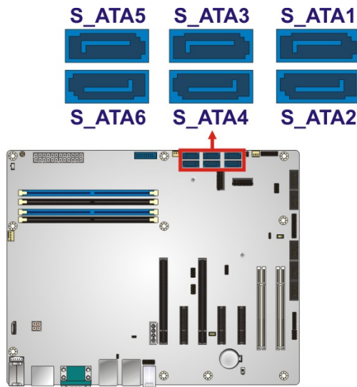
Figure 3-24: SATA 6Gb/s Drive Connector Locations
