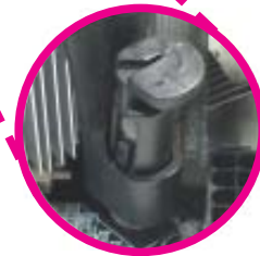
"Unlocked" position of push-pin
