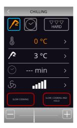
Set the desired value using the key. Once set-up is complete press the next to the edited value and return to the previous screen.
