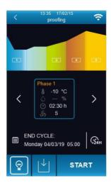
The cycle starts up when the START area is pressed and it terminates automatically at the end of phase 4 and according to the date and time set for it to end, at which time a buzzer sounds.
