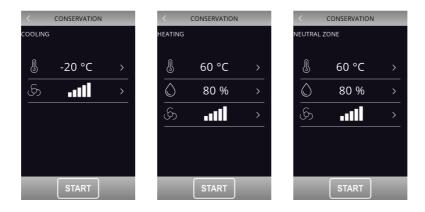
The cycle starts when the START area is pressed and remains active until the STOP area is pressed.
