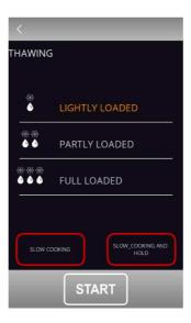
To make it easy, the quantity of product to be selected is divided into three load bands for each of which the controller will load three different sets of parameters, according to the following framework.
