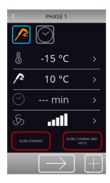
The customized cycle starts up and activates the first phase, which by default is a needle probe phase. It is possible to change the probe phase to a time controlled phase and to set the relative set points.
