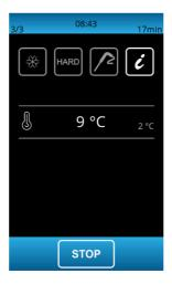
The conservation phase is not timed and is only terminated when the stop key is pressed.
