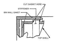
**NOTE**. Bin wall gasket must be cut to clear the stiffener ends as shown on drawing. Do not put any stiffeners crossing the ice drop opening.
