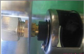
5. The standard setting for the air shutter must be FULLY open. However, the air shutter can be adjusted according to the actual flame, to eliminate yellow tipping or other burner problems which is caused by too much air or lack of air.
