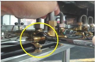
Remove the front main burner injector, and replace the injector with the appropriate orifice size for the new gas type to be used. Refer to the GAS SPECIFICATION Table on Page 21, for the main burner injector orifice size. Use 13mm spanner to remove and install the injector.
