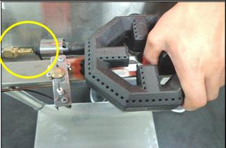
Pull-out all the burners from the injector and replace as necessary.
