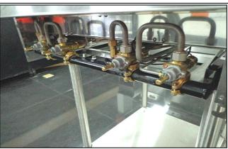
6. For the front main burner injector, remove the front control panel cover.
