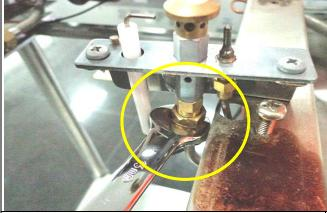
Reconnect the pilot pipe assembly to the pilot injector of the FDS. Use 13mm spanner.
