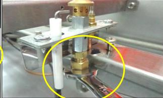
10. Re-install the FDS and its mounting screws.
