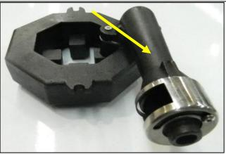
Loosen the screw and move the air shutter to close or open.
