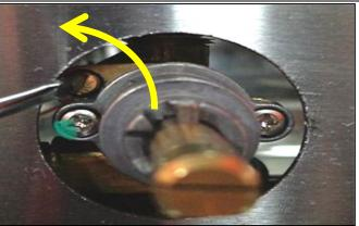
18. When LPG is used, the installed low flame adjustment screw must be Ø0.7mm. From the FULLY closed position, open the adjustment screw by about 90°, by turning it counterclockwise to open.
