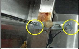
Re-install the old pilot injector to the new FDS or replace the pilot injector with a new one, if you deemed it necessary. Use 10mm spanner. It is also recommended to clean the pilot injector by blowing in air before reinstalling it.
