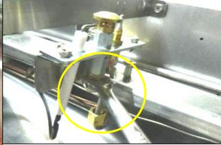
6. Remove the pilot injector from the FDS. Use 10mm spanner.
