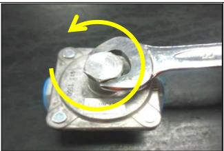
19. Remove the gas regulator from the equipment. Then, open the gas regulator cap. Use 22mm spanner.
