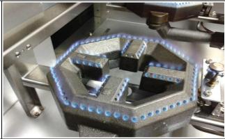
. Turn the screw clockwise to decrease the flame height/strength. When the screw is tight, stop rotating as this could damage the screw. It also means the adjustment is already at its minimum height.
