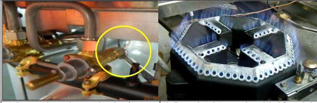
11. Reconnect the new thermocouple to the safety gas valve. Use 9mm spanner. Tighten the thermocouple up to 2.5N-m of torque. Tightening too much can cause the thermocouple to break and fail.
