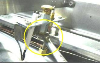
12. Remove the pilot injector from the FDS, and replace with the appropriate orifice size for the new gas type to be used. Refer to the GAS SPECIFICATION Table on Page 21, for the pilot injector orifice size. Use 10mm spanner to remove and install the pilot injector.
