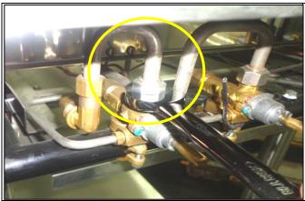
7. Loosen the fitting of the front burner main pipe assembly connected to the gas valve. Use 19mm spanner.
