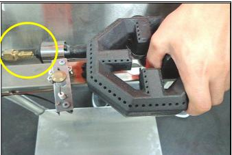
4. Pull-out all the burners from the injector.
