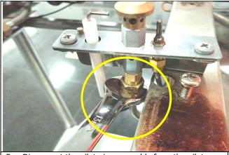
5. Disconnect the pilot pipe assembly from the pilot injector of the FDS. Use 13mm spanner.
