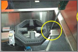
3. Remove the burner lock screw/s.
