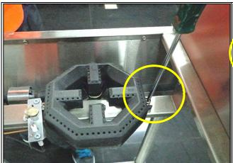
3. Remove the burner lock screw/s.
