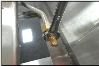
5. Remove the rear main burner injector, and replace the injector with the appropriate orifice size for the new gas type to be used. Refer to the GAS SPECIFICATION Table on the succeeding page. Use 13mm spanner to remove and install the injector.
