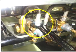
After installing the new main burner injector, rotate the main pipe assembly back to its original position and tighten the connection fitting. Use 19mm spanner.
