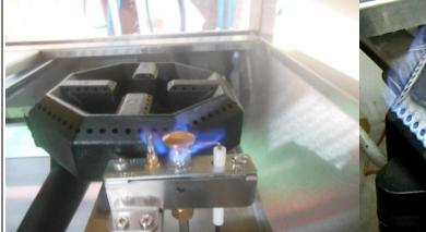
9. Turn on the isolation gas valve and light up the pilot and check if the flame hits the tip of the thermocouple. Adjust the thermocouple by moving upward or downward, or adjust the pilot head, so that the flame hits the tip.
