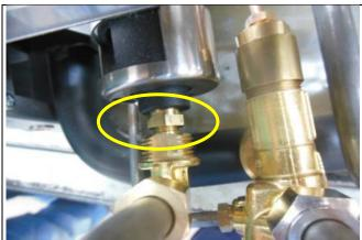
11. Install back the burner. When installing the burner to the injector, make sure that the injector is fully inserted in the burner hole and that the injector is properly aligned. Misalignment of the injector into the burner hole can cause yellow tipping of flames.
