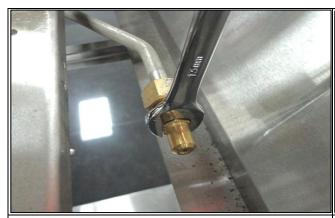
Remove the rear main burner injector, and replace the injector with the appropriate orifice size for the gas type. Refer to the GAS SPECIFICATION Table on page 21. Use 13mm spanner to remove and install the injector.
