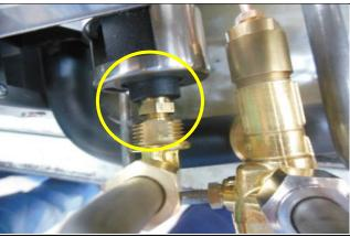
6. When installing the injector into the burner, ensure that both are aligned with each other. Misalignment can cause yellow tipping of flames and sooting.
