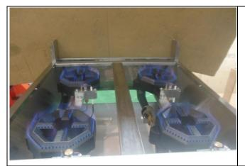
25. Check for gas leaks. Use soapy water (bubble test) to check for leaks. Never use naked flame to check for leaks. Then, open the burners and perform a function test.
