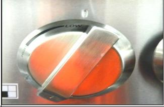
3. Put back the knob. Turn ON the burner and set the knob to low flame.
