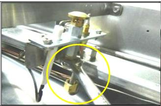
5. Remove the pilot injector from the FDS.
