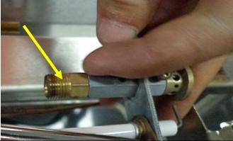
Re-install the old pilot injector to the new FDS or replace the pilot injector with a new one, if you deemed it necessary. Use 10mm spanner. It is also recommended to clean the pilot injector by blowing in air before reinstalling it.
