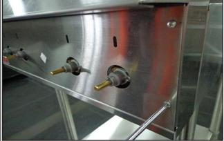
5. Return the control panel. Turn ON the isolation gas valve and check for gas leaks on the part replaced.
