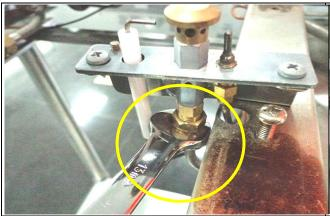
11. Disconnect the pilot pipe assembly from the pilot injector of the FDS.
