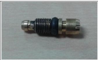
16. Replace the low flame adjustment screw with the correct type according to the gas type used. Use Ø0.7mm for LPG and Ø1.6mm for NG. Refer also to the Gas Specification table. Then, set the adjustment screw.
