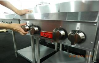
Remove the knob/s of the burner that needs to be adjusted..
