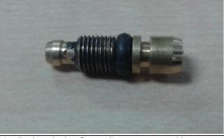
Replace the low flame adjustment screw with a Ø0.7mm hole for a wider range of low flame adjustment. Make sure that the adjustment screw is hand tight after installation.
