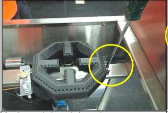
3. Remove the burner lock screw/s.
