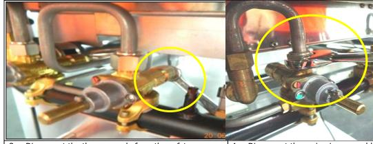
3. Disconnect the thermocouple from the safety gas valve. Use 9mm spanner.
