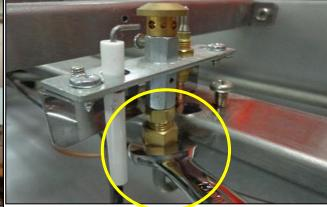
. Disconnect the pilot pipe assembly from the pilot injector of the FDS. Use 13mm spanner.
