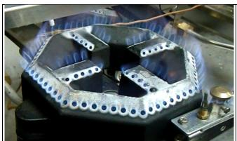
Turn the screw counter-clockwise to increase flame height/strength. Stop rotating when the flame stops increasing its height. It means it has already reached its maximum height.
