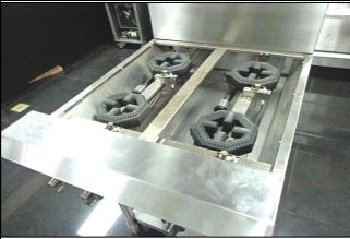
Remove the trivets and knobs.
