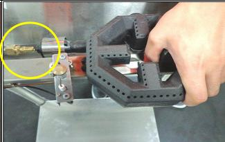
Pull-out all the burners from the injector and replace as necessary.
