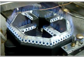
After burner installation, turn on the isolation gas valve and light the burner and check if it has blue flame. Adjust the air shutter as necessary. Otherwise, follow the troubleshooting guide.
