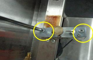
6. Remove the two mounting screws of the FDS.
