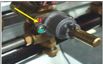
Remove the low flame adjustment screw from the safety gas valve. Use a small screwdriver, and turn counter-clockwise, then use a pair of pliers to pull it out from the gas valve.
