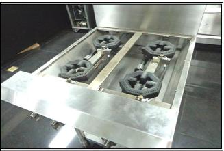
Remove the trivets and knobs.
