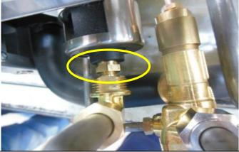
14. When installing the burner to the injector, make sure that the injector is fully inserted in the burner hole and that the injector is properly aligned. Misalignment of the injector into the burner hole can cause yellow tipping of flames.
