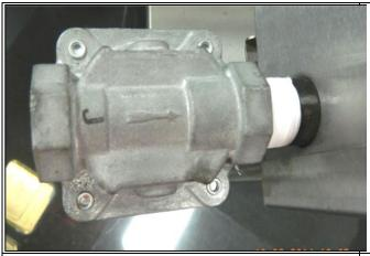
23. Install the gas regulator to the unit. Ensure that the arrow points toward the appliance. The arrow signifies the flow of the gas.
