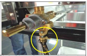
Install the new safety gas valve to the main gas pipe manifold. Use 10mm spanner to install the mounting bolts.
