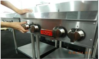
6. Once the low flame is set, check the bypass screw for gas leak, as you might have opened the bypass screw too much. Use soapy water to check for gas leak on the bypass screw. Then, return the knob/s after the gas leak test.
