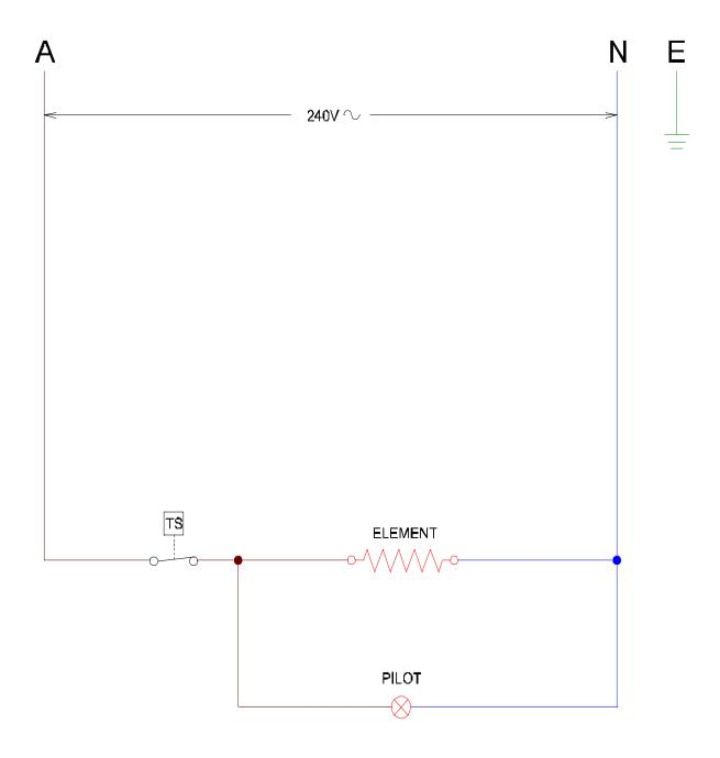
**Note:** This circuit diagram has been provided for reference and to assist qualified service and repair agents only. Under no circumstances should persons not suitably qualified attempt repairs to any electrical equipment.
