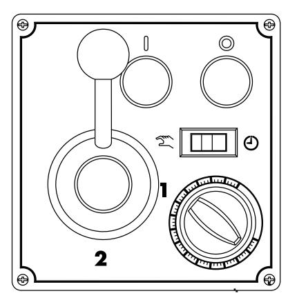
All models are furnished with two button-switches, which control power to the mixer.
