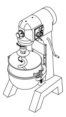
BE SURE TO CHECK MIXING ROTATION WHEN ELECTRICAL CONNECTS ARE IN PLACE FOR ALL THREE (3) PHASE RIGGING.
