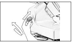
2. If the knife cover is tight, loosen it with pressure on the tension rod knob.
