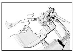
Press the deburring button and keep it pressed for 2-3 seconds;
