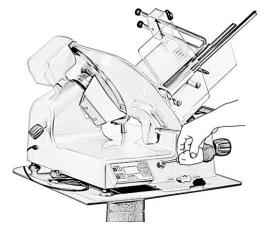
7.4 Lubricating the transversal guide rods of the table and food press (weekly)
