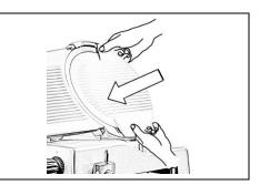
2. Insert the tie rod for locking and screw completely.
