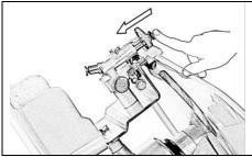
9. Pull the fixing sharpener knob in order to unhook the sharpener from the sharpening position and turn the body, as shown in the picture.
