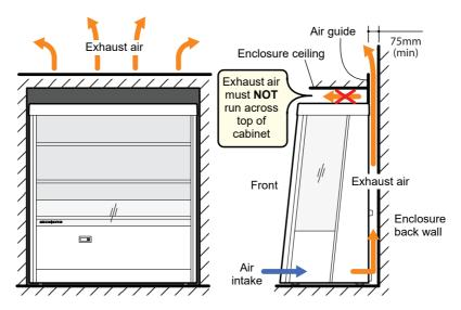
**Enclosed installation ventilation requirements**
