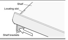
Optional When the chiller is ordered with the optional gravity feed matting, each shelf Gravity Shelf is supplied with corresponding gravity feed matting and shelf dividers. The System gravity shelf system comes in three sizes to suit the three different size shelves.
