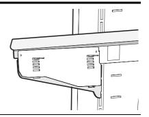
2. Sit the corresponding metal shelf on the cantilevered brackets ensuring the back of the shelf clips over the rear of the brackets.
